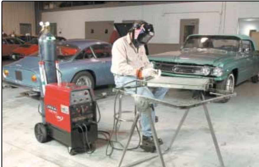
AC Auto-Balance is especially useful on critical aluminum applications.
