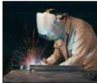
Conventional CV short circuit transfer using CO 2 and .045" solid wire.
