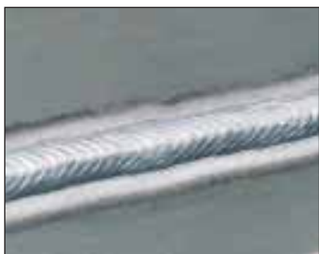
Pulse-On-Pulse on 3 mm Aluminum
