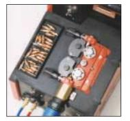
are equipped with the same rugged four-roll drive system. This drive is easy to access and protected by the unique fliptop cover. The wire guidance from the coil to gun tip is smooth and accurate. It is designed to eliminate tangles and guarantee trouble free feeding.
