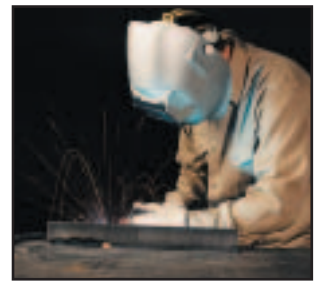
STT using CO 2 and .045" solid wire. Note reduced spatter and fume.
