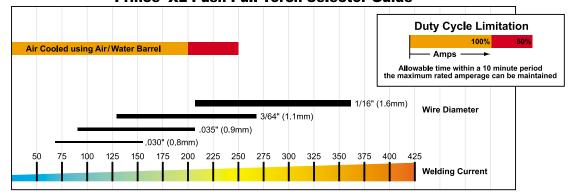
**NOTE:** Wire Diameter and Current may vary depending on your particular Power Supply and Welding Voltage. Wire Diameter and Current based on 5356 Aluminum Wire.
