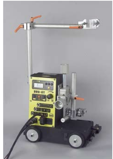
The BUG-GY can weld lap joints with a minimum height of 3/8" (9.53 mm).
