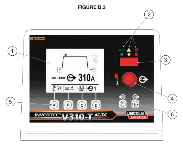
The V310-T AC/DC User interface consists of the following (Refer to Figure B.3):
