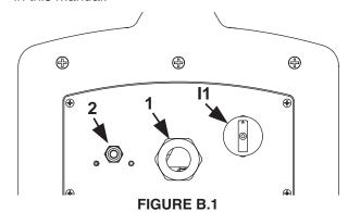
\* 1 : Supply cable \* 2 : Gas attachment I1 : Power Switch
